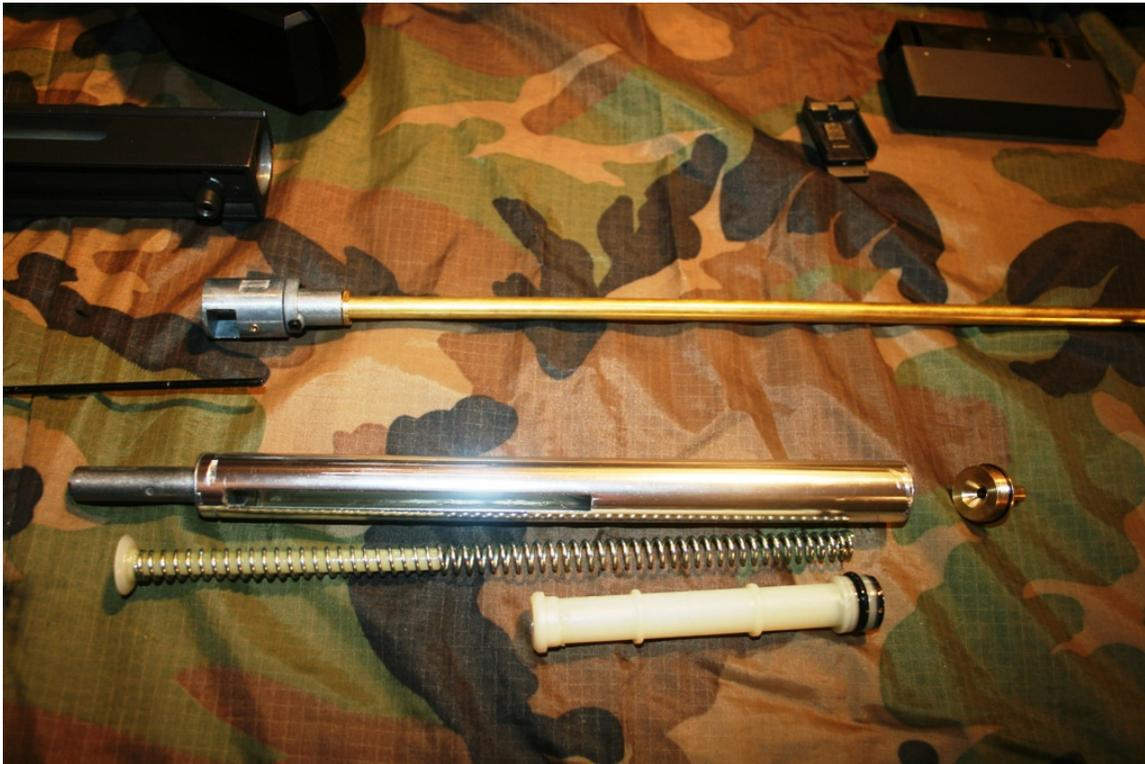
The hopup chamber is made out of metal and seems to do its job. The hopup rubber though is made out of low quality rubber. Unfortunately without modification you can not put standard AEG or VSR type hopup rubbers into this rifle. The only other upgrade hopup replacement is the PDI Type 96 hopup chamber.
